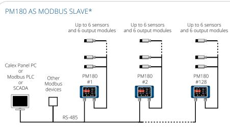
Each PM180 is a slave device on the main network and the master on each network of sensors. Up to 128 PM180 units can be connected to the same Modbus Master. This layout allows hundreds of sensors to be connected in a network.
